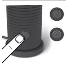
4. Place the lid on the Aeroccino. For a hot preparation, briefly press button to start. Button lights up Red. Take approx. 70–80 sec. For cold milk froth, keep button pressed for approx. 2 seconds. Button lights up Blue. Takes approx. 60 sec.
